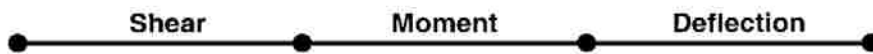
Figure A.17. Hypothetical series system model of typical girder (Estes and Frangopol 2001).
